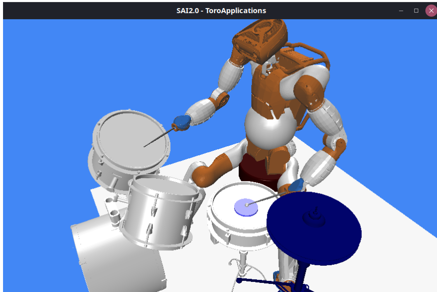
Figure 8: Collision objects on the drum and Toro's hand were added and collision checking incorporated.
